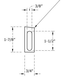
NOTE: TOP RAIL TENONS ARE <u>NOT</u> PERFECTLY IN THE CENTER. THEY ARE PUSHED DOWNWARD. 1/4" FROM THE TOP AND 1/8" FROM THE BOTTOM. 3/16" FROM LEFT AND RIGHT SIDES.
